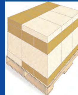
Half-Size Configuration: 10 Boxes Per Tier Box Dimensions: 398 mm x 298 mm, or 15½ in. x 11½ in.
